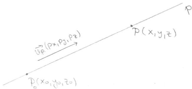
$$\begin{aligned} X &= \begin{bmatrix} x_0 \\ y_0 \\ z_0 \end{bmatrix} + t \cdot \begin{bmatrix} p_x \\ p_y \\ p_z \end{bmatrix}, \quad t \in \mathbb{R} \\ Y &= \\ Z &= \end{aligned}$$
