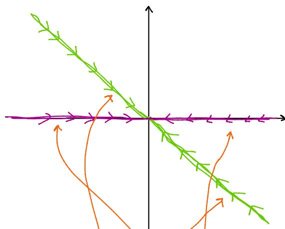
$$c_1 = 0, \quad x(t) = \begin{bmatrix} e^{-3t} \\ -e^{-3t} \end{bmatrix}, \quad x_2 = -x_1 < 0$$
